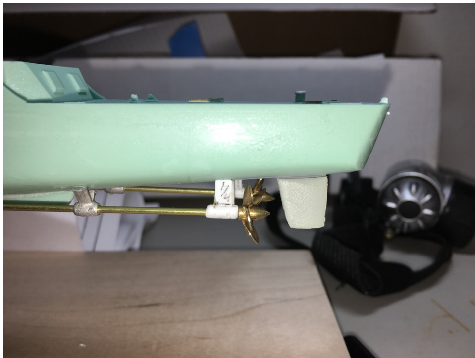
Figure 4. Propeller shafts and rudders installed.
