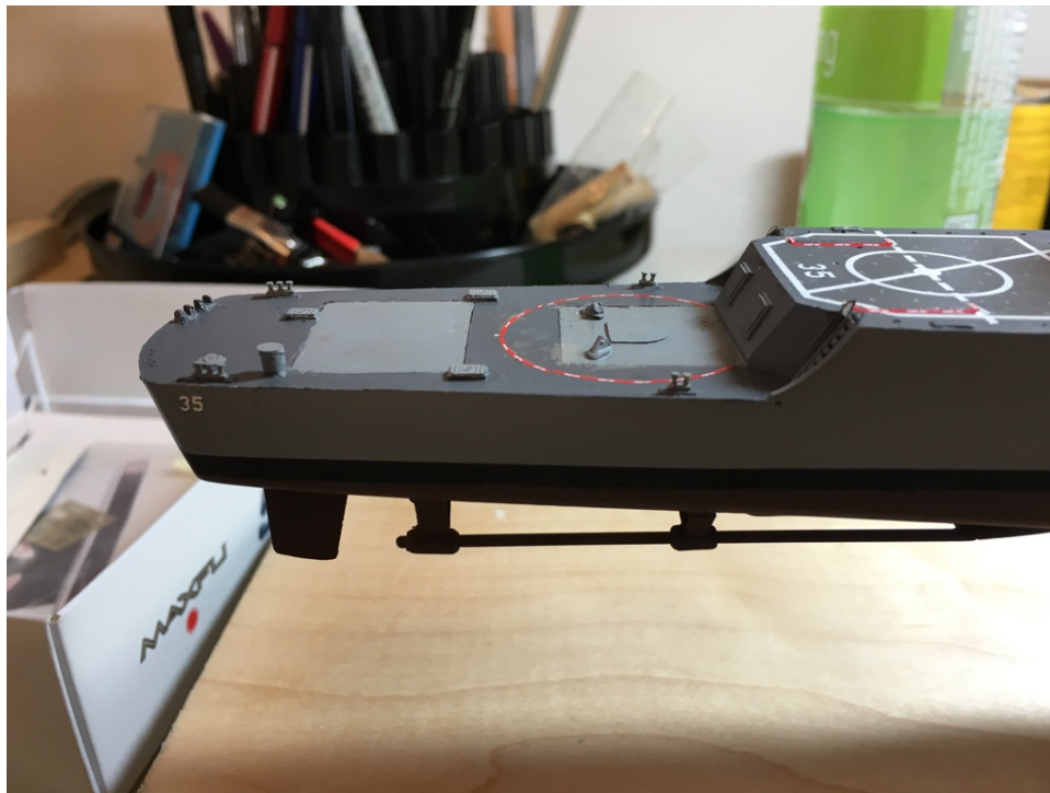
Figure 15. Note the addition of bitts for mooring lines.
