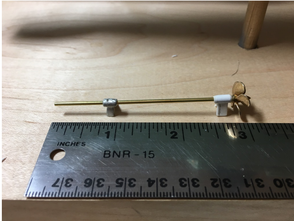
Figure 3. The custom-built port shaft with screw.
