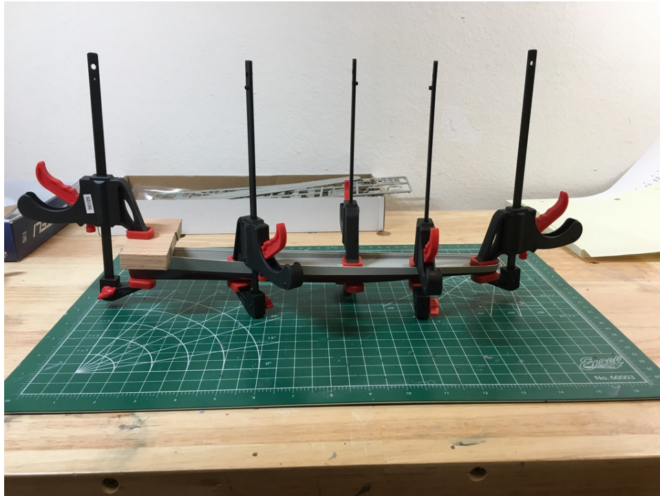
Figure 3. Gluing the Upper and Lower Hull Together.
