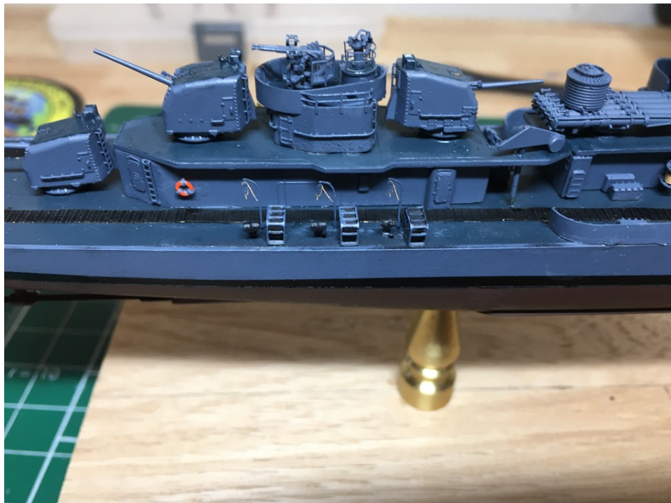
Figure 28. Starboard K-guns, Storage Racks and Loading Davits.
