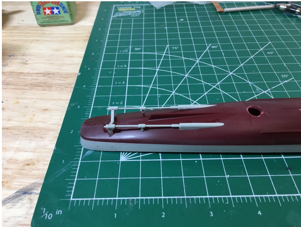
Figure 5. Propeller Shafts are Built. Note the Mounting Hole.
