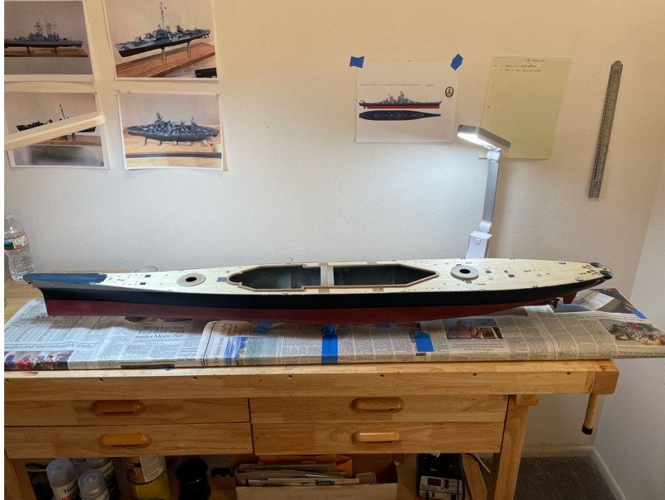
Figure 10. The Main Deck Veneers are in Place.
