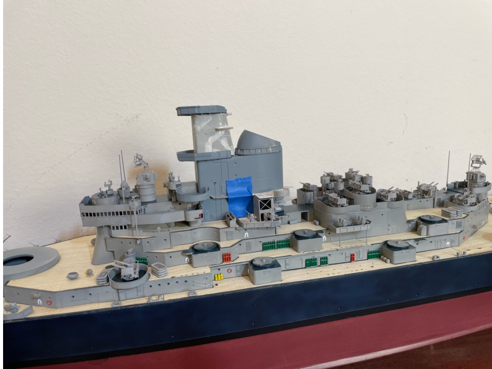
Figure 42. Dry Fit for Spot 1 and the Forward Stack. The Discolored Parts are Salvaged from Missouri-1.
